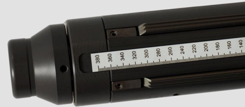
Pneumatic expanding shafts with axial movement are the most suitable solution to unwind and rewind coils in cantilever applications. The axial movement of the shaft allows the coil to be aligned without removing it from the shaft itself.
